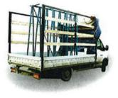
All-metal stand structure firmly connected to the loading surface of the delivery low-floor type of vehicle.
