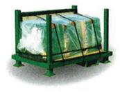
Returnable metal stand for the transportation of products from the processing of furniture glass (mirrors, float and ornamental glass, etc.). Two types differing in length (1,250 or 1,550 mm). They have an "L" shaped profile, where the bottom and work rest are made of plywood.
